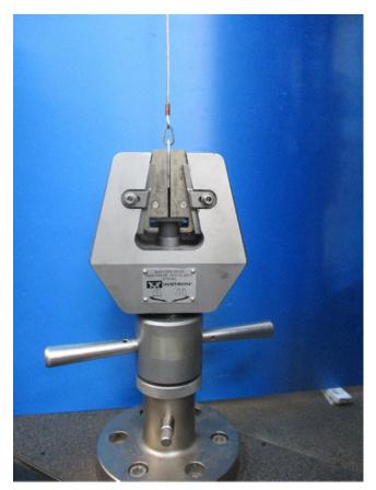
Figure 6.4: Measuring the strength of the breakaway clip in the straight configuration.
