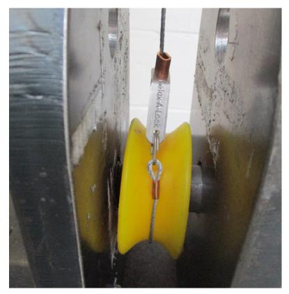
Figure 3.3: Snare loop on plastic spool mounted in clevis arrangement.
