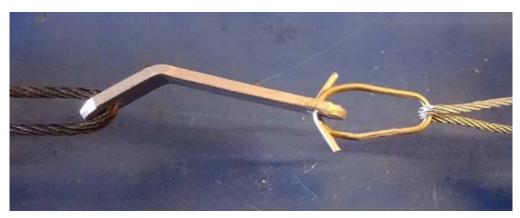
Figure 6.1: Configuration employed in the tests to measure the breaking strength of the breakaway clip undertaken for Perdix (from [4]).
