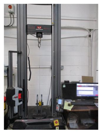
Figure 3.1: INSTRON tensile testing machine with DB snare mounted ready for testing.
